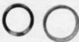
OVERSIZE VALVE SEAT INSERTS FOR 1956-58 GOLD STAR
