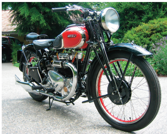
This 1939 600cc Square 4 was restored and photographed by Terry Barber. The 600cc pushrod engine is quite rare, having been made only in 1939 and 1940. (Photo courtesy of AMCNA)
